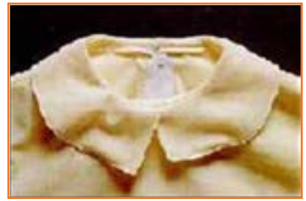
Fig.3.1.22(c): Interlining shrinking
