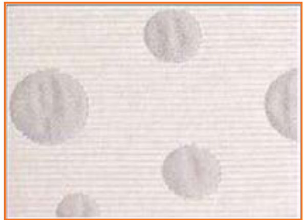
Fig.3.1.26(b): Fusing delamination
