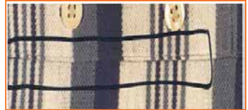
Fig.3.1.17: Marker Making Defects
