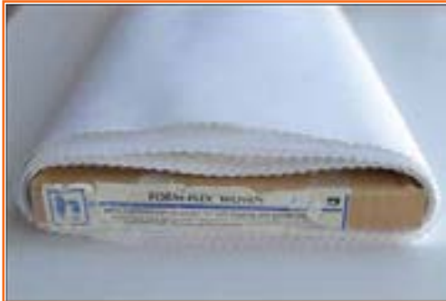
Fig.2.1.73: Nonwoven Non-fusible Backing Paper
